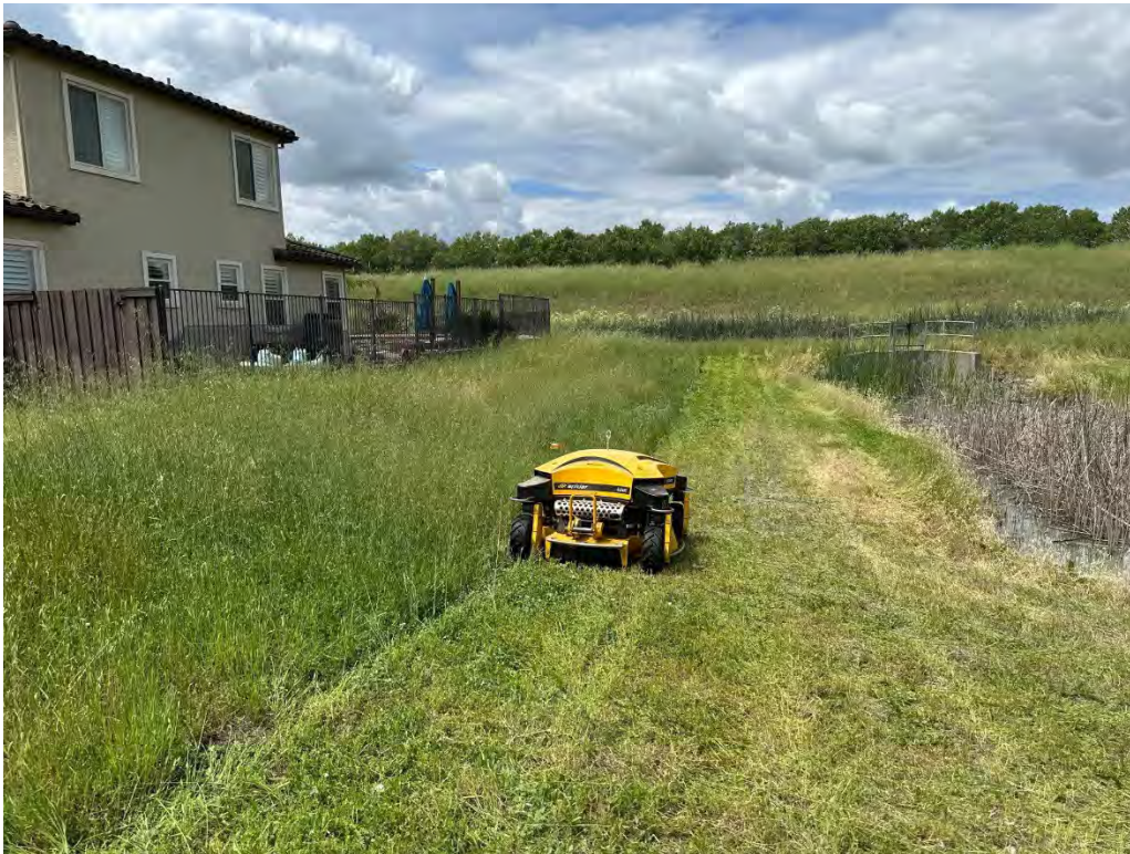
Remote mower cutting grass along canal
